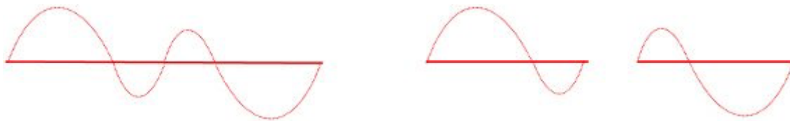
Figure 4 - Real wavecycle (left) consisting of two pseudo-wavecycles (right)
